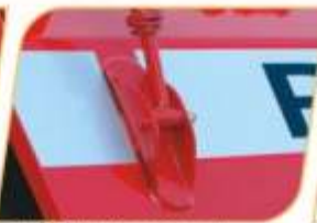
Central & Offsettable positions with clevis mounting plates adjustable on a round tube
